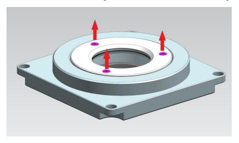
Remove the filter and rubber o-ring from pocket.
