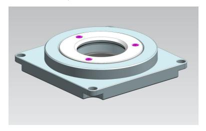
Unscrew three M1.6 screws using TX5 screwdriver and remove the holding ring.
