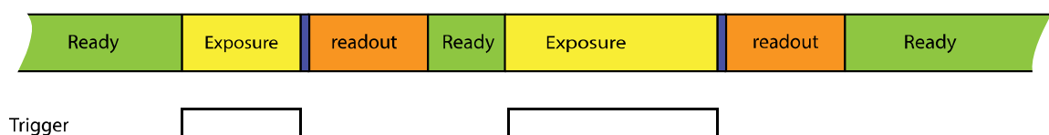
figure 4-5, Exposure defined by trigger pulse length
