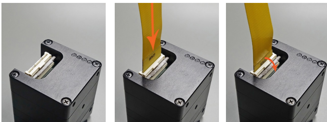
figure 3-47 MX X2G2 FPC insert procedure option -FV
