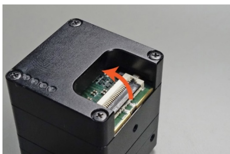
figure 3-43, MC FPC cable CBL-PCIEFLEX-X2G2-xxx ends
