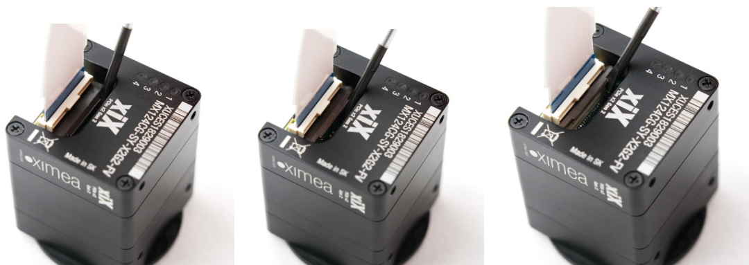
figure 3-46 MX X2G2 unlocking the connector (option –FV)
