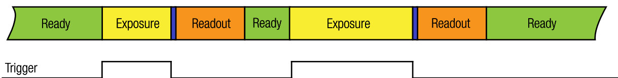
Figure 53: Exposure defined by trigger pulse length
