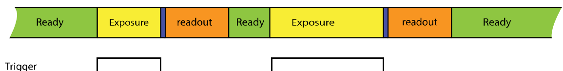
figure 4-7, Exposure defined by trigger pulse length
