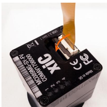
figure 3-47 MC FPC insert procedure option -FV
