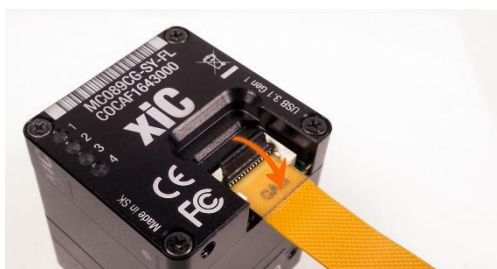
figure 3-45, MC FPC insert procedure option -FL
