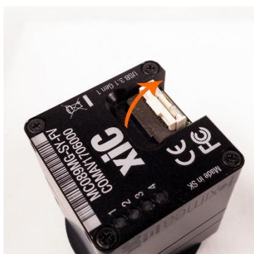
figure 3-46, MC FPC detach procedure option -FL
