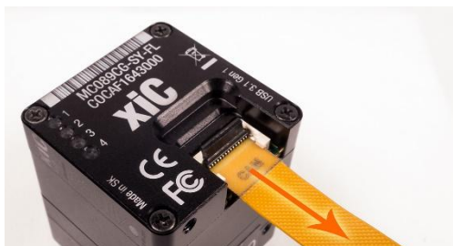
figure 3-46, MC FPC detach procedure option -FL
