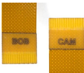
figure 3-41, FPC cable CBL-MQ-FL-xxx laser marking
