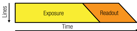
Figure 60: Global reset release mode - schematic
