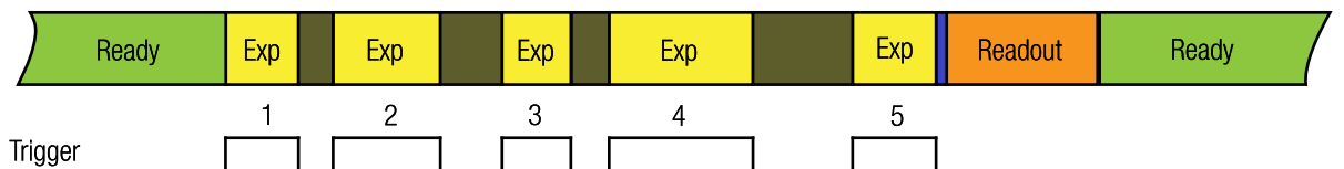
Figure 56: Multiple exposures - exposure time defined by trigger pulse length - number of exposures set to 5
