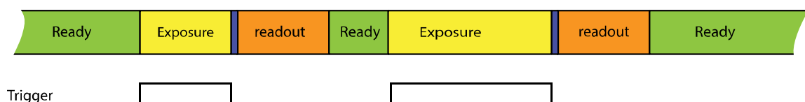
figure 4-6, Exposure defined by trigger pulse length
