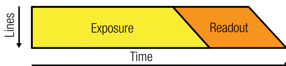
Figure 39: Global reset release mode - schematic
