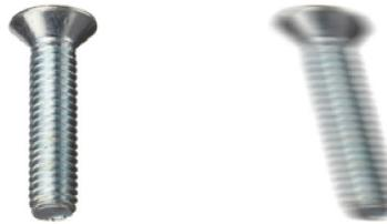
Figure 50: Rolling shutter mode image of a horizontally moved object, long exposure time
