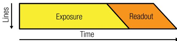
Figure 45: Global reset release mode - schematic
