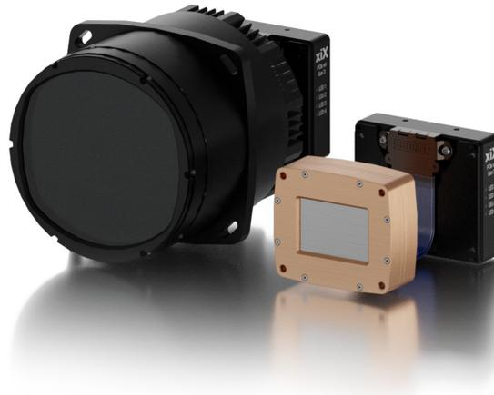
The CMOS cameras are equipped with a PCI-Express interface allowing data throughputs up to 32 Gbit/s. The separation of the sensor head from the camera body can further assist with building various multicamera systems.
