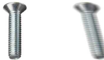
Figure 47: Rolling shutter mode image of a horizontally moved object, long exposure time
