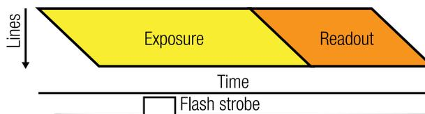
Figure 85: Rolling shutter mode with flash - schematic
