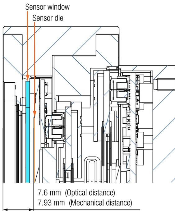
Figure 15: Cross section of MX1018xR-SY-X4G3-FF camera models
