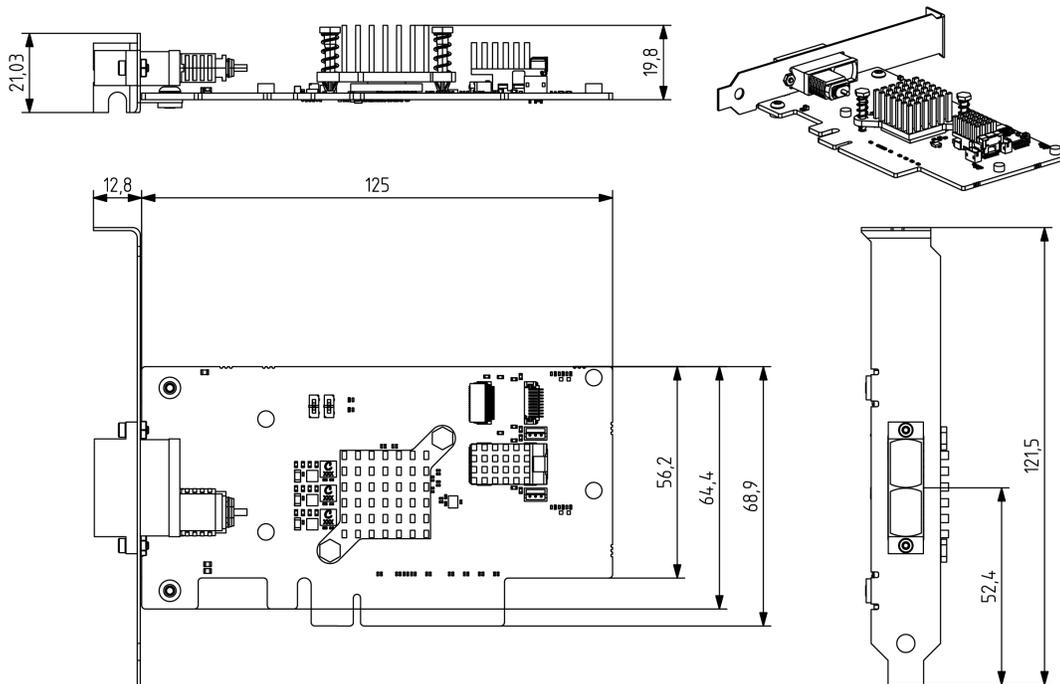
Figure 72: Dimensional drawing of host adapter HA-1P-X4G3-MTP-X8G3
