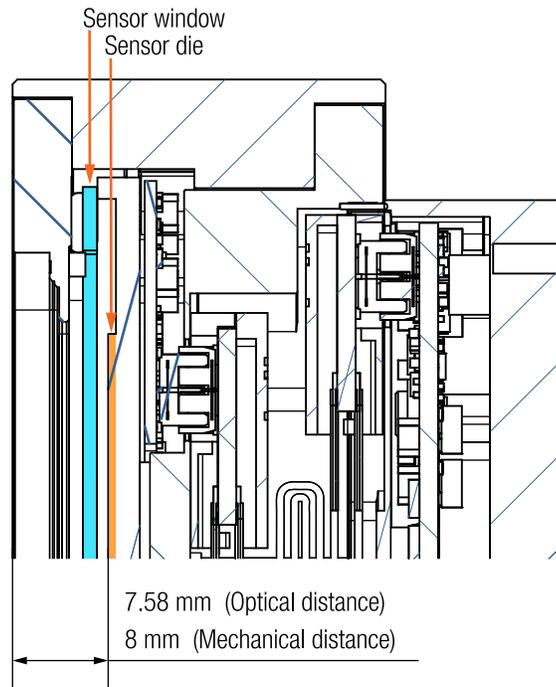
Figure 17: Cross section of MX2457xR-SY-X4G3-FF camera models
