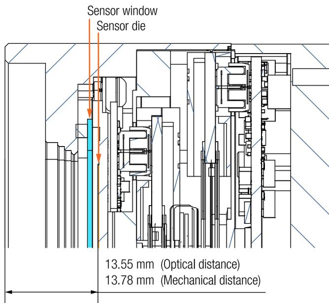
Figure 18: Cross section of MX610xR-SY-X4G3-FF camera models
