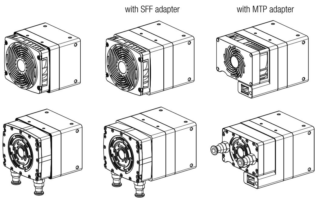
Figure 6: Camera with accessory & cooling options
