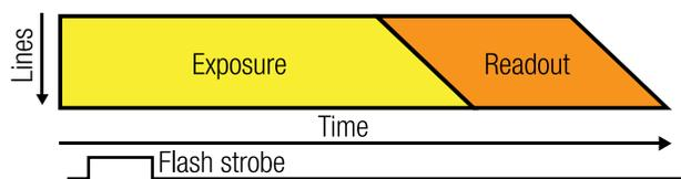
Figure 81: Global reset release mode with flash - schematic
