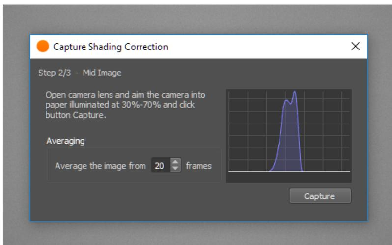
Figure 89: Flat field correction - Mid- saturated image
