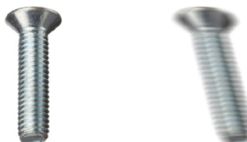
Figure 84: Rolling shutter mode image of a horizontally moved object, long exposure time
