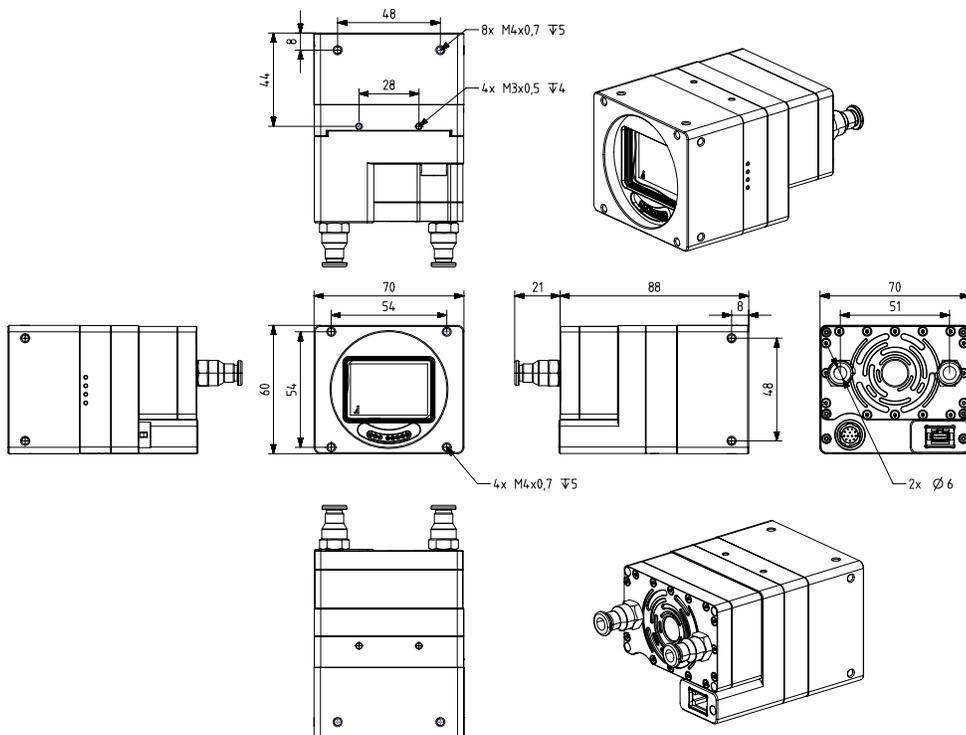
Figure 59: MX610xR-SY-X4G3-FF with MTP adapter and water cooling
