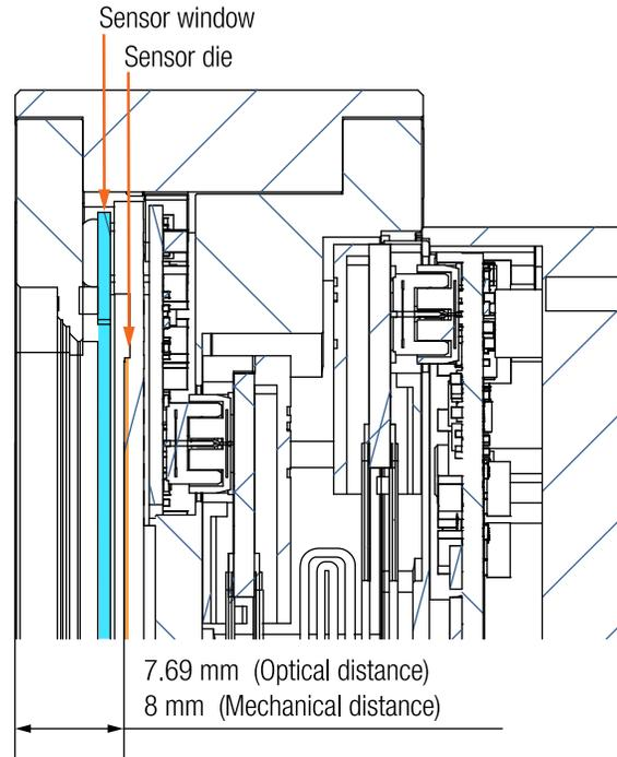
Figure 16: Cross section of MX1510xR-SY-X4G3-FF camera models
