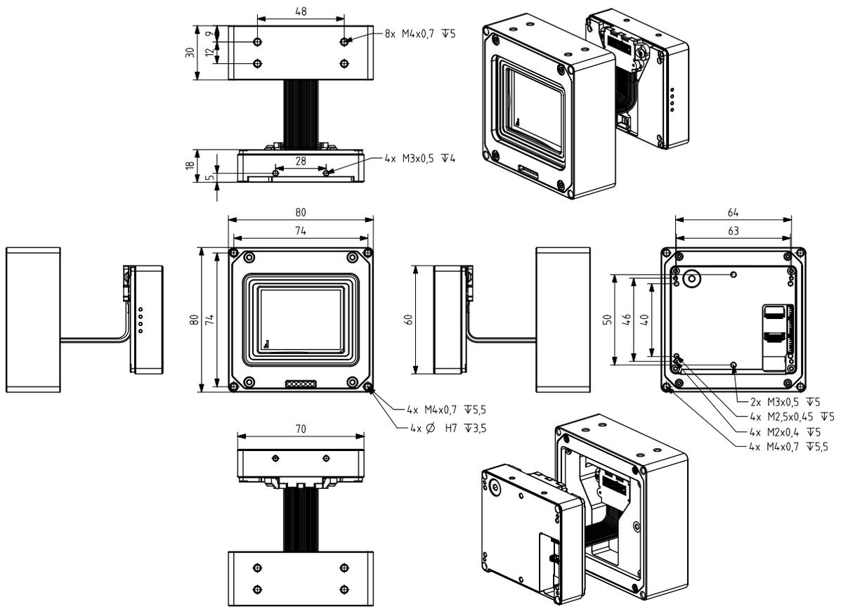
Figure 27: Dimensional drawing of MX1018xR-SY-X4G3-FF with detached sensor sub-assembly
