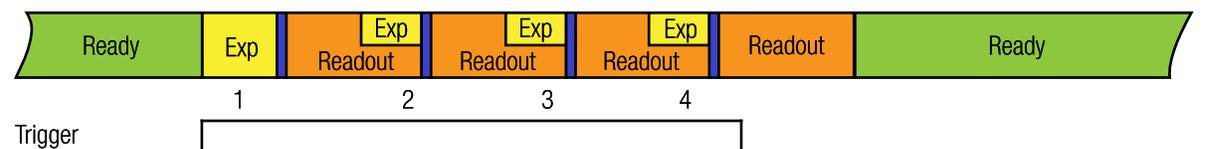
Figure 77: Triggered burst of frames – frame burst active
