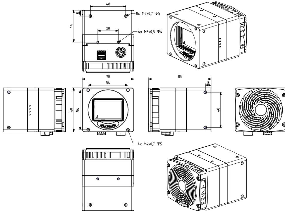
Figure 65: MX610xR-SY-X4G3-FF with SFF adapter and fan cooling
