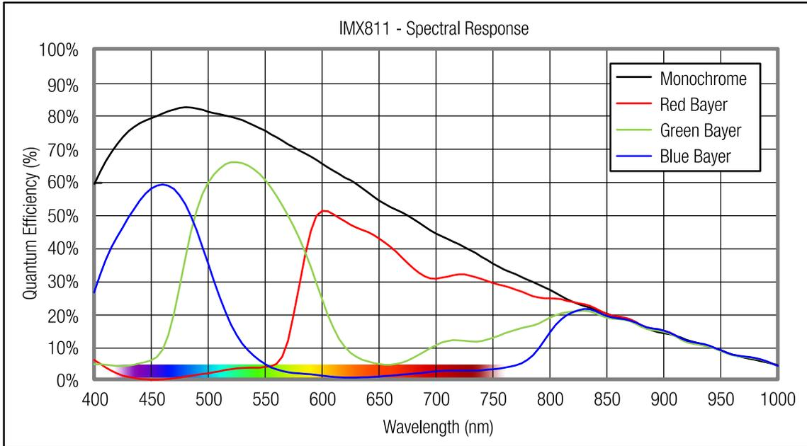
Figure 21: Graph quantum efficiency of Sony IMX811
