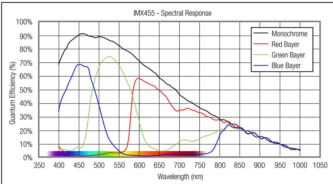
Figure 22: Graph quantum efficiency of Sony IMX455
