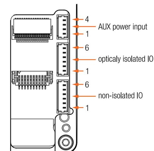
Figure 34: IO connectors position
