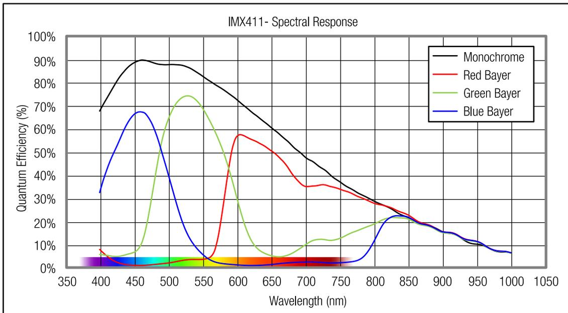
Figure 20: Graph quantum efficiency of Sony IMX411
