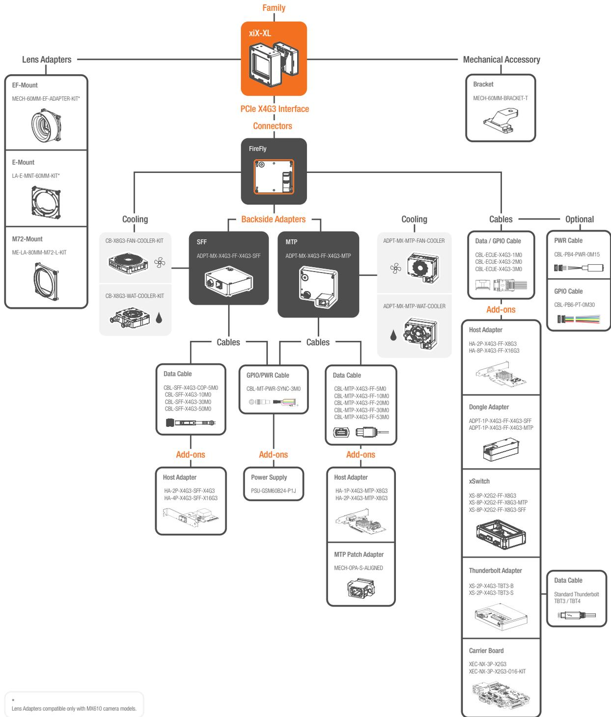
Figure 7: Diagram of accessories and specific connections for the xiX-XL camera family
