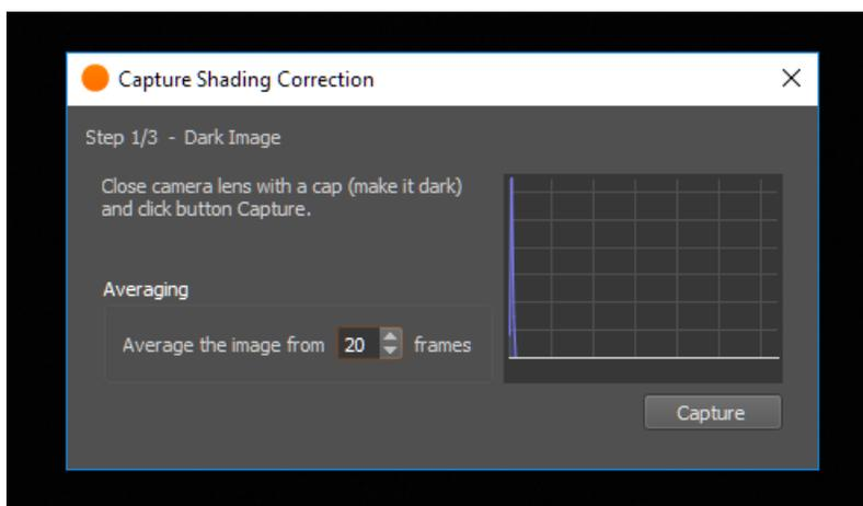
Figure 88: Flat field correction - Dark image
