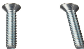
Figure 70: Rolling shutter mode image of a horizontally moved object
