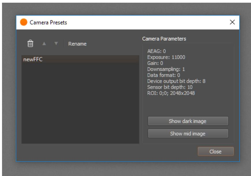
Figure 92: Flat field correction - FFC management
