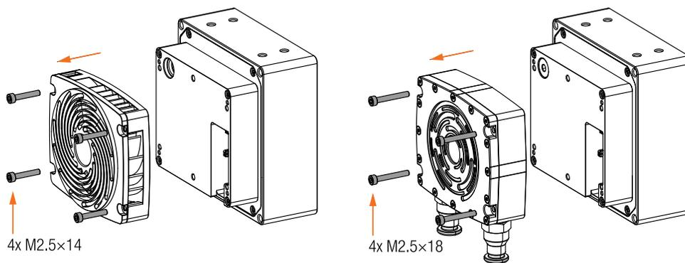
Figure 42: Detaching heatsink
