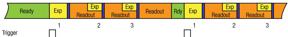
Figure 76: Triggered burst of frames – frame burst start
