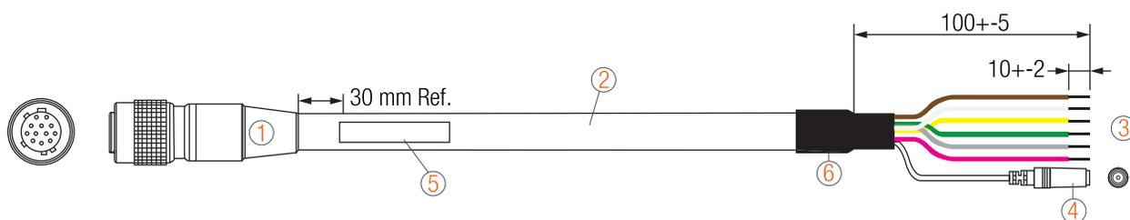
Figure 60: CBL-MT-PWR-SYNC-3M0 drawing
