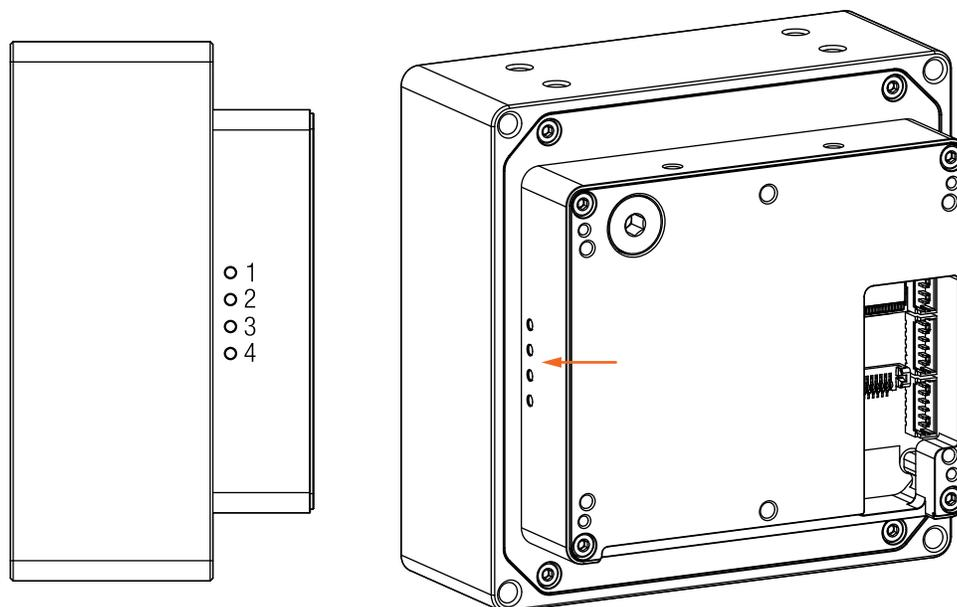
Figure 31: Position of LEDs on xiX-XL camera
