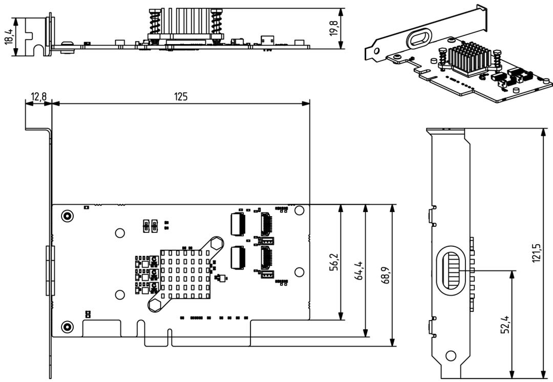
Figure 74: Dimensional drawing of host adapter HA-2P-X4G3-FF-X8G3
