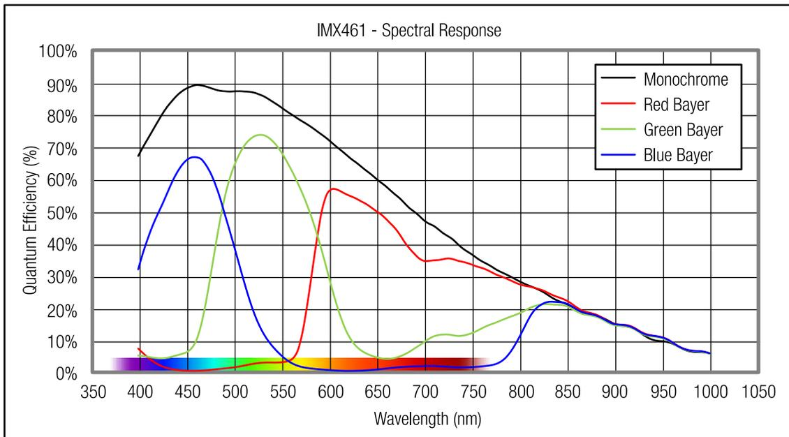
Figure 19: Graph quantum efficiency of Sony IMX461
