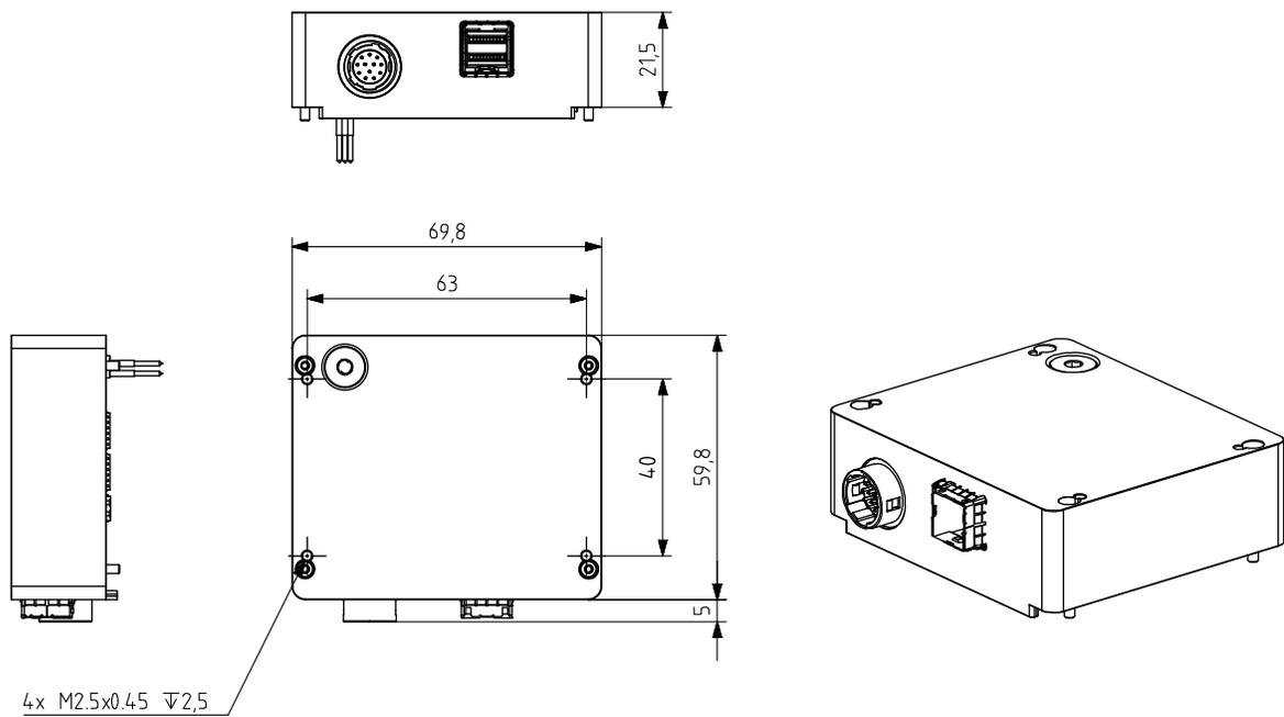
Figure 63: ADPT-MX-X4G3-FF-X4G3-SFF dimensional drawing
