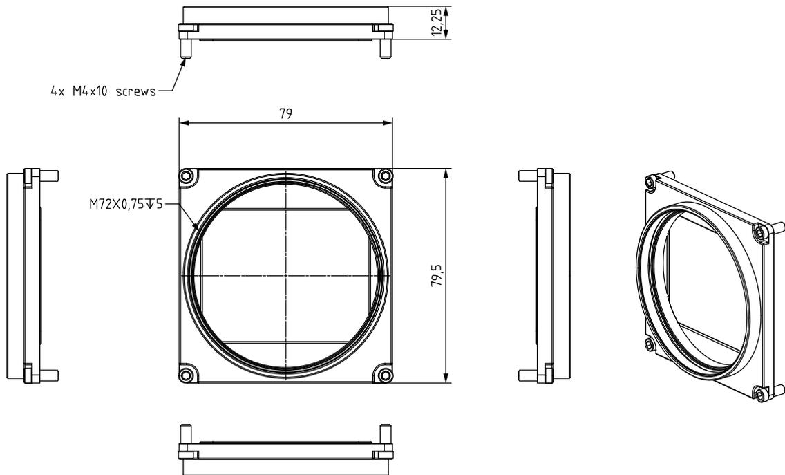
Figure 55: Dimensional drawing of ME-LA-80MM-M72-L
