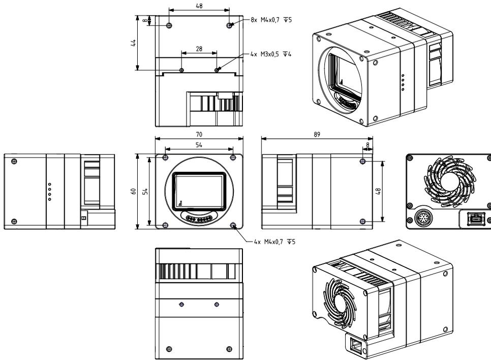
Figure 58: MX610xR-SY-X4G3-FF with MTP adapter and fan cooling
