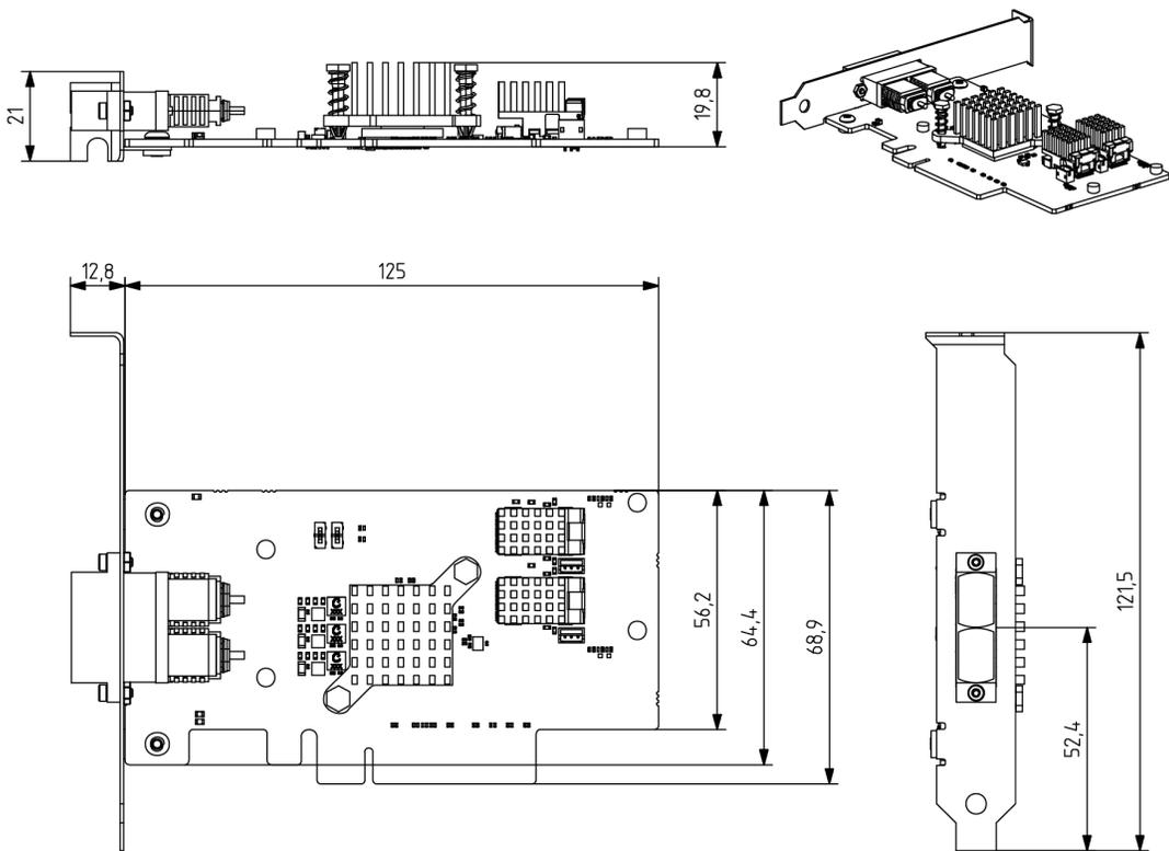
Figure 73: Dimensional drawing of host adapter HA-2P-X4G3-MTP-X8G3
