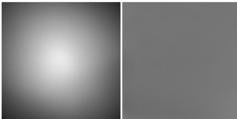
Figure 86: Flat field correction - images comparison
