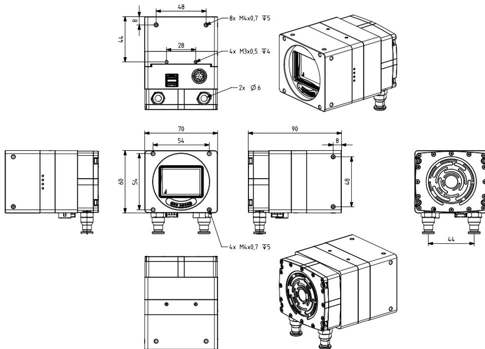
Figure 66: MX610xR-SY-X4G3-FF with SFF adapter and water cooling
