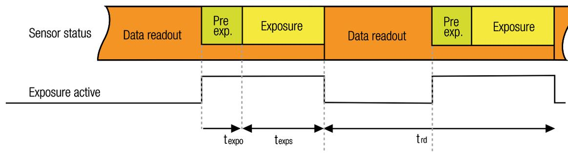
Figure 75: Acquisition mode - free run
