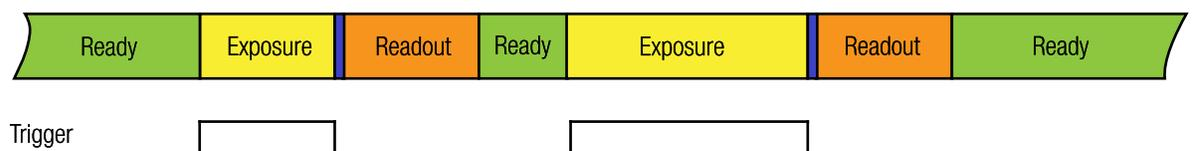
Figure 78: Exposure defined by trigger pulse length
