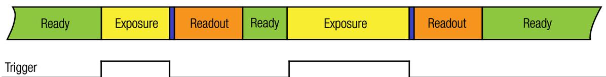
Figure 63: Exposure defined by trigger pulse length
