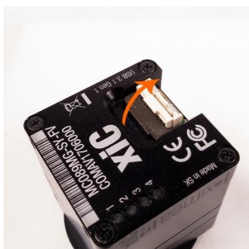
figure 3-46, MC FPC detach procedure option -FL
