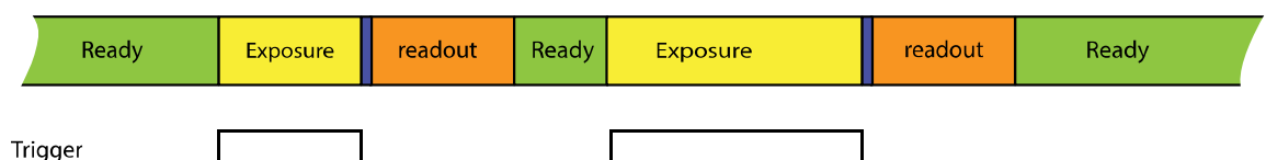
figure 4-7, Exposure defined by trigger pulse length
