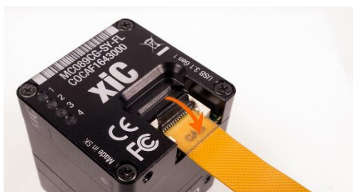
figure 3-45, MC FPC insert procedure option -FL
