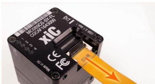
figure 3-46, MC FPC detach procedure option -FL
