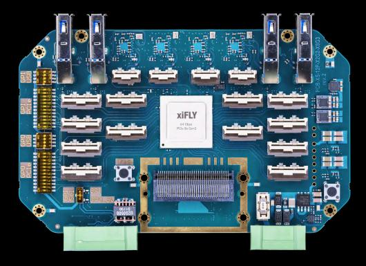
An example of a standard xiFLY component, xiSwitch module with 8x USB3 and 12x PCIe X2G2 camera ports and single PCIe X8G3 host iPass port for total image data throughput of 64 Gbps.
