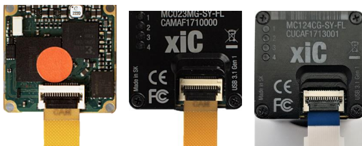
Figure 6-5, xiQ (left) and xiC (right) – camera side, correct FPC cabling
