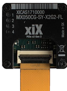
Figure 3-3, xiX X2G2 – camera side, correct FPC cabling
