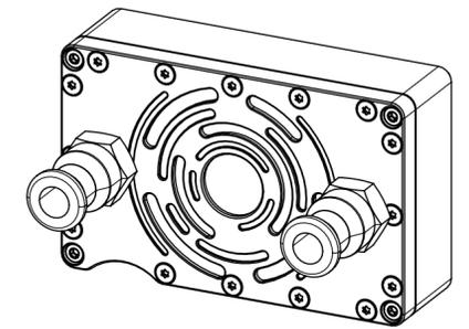
\* Designed for 6mm (water rated) tubes
